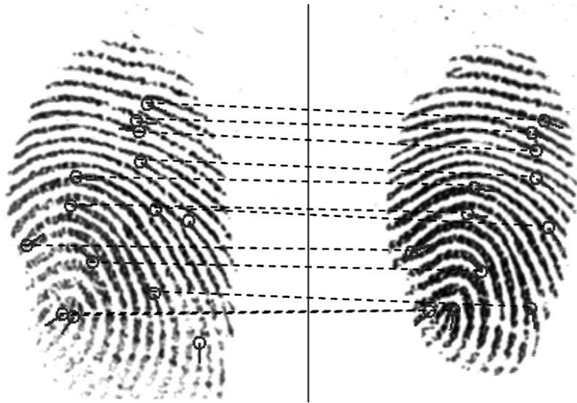
Fig. 11. Match two fingerprints is equivalent to find the corresponding links between feature points.
