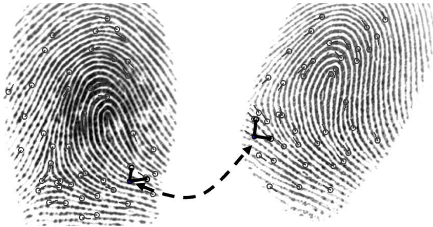
Fig. 7. An example of two false matched secondary features. They are similar at the local structures but conflict with each other in global context (at very different locations with respect to the core and delta points).
